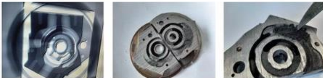
Figure 3: Residual sand inside the water channel after X-ray analysis and in the real turbocharger body section
