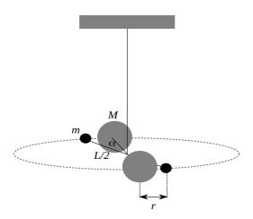
Figure 11.1: Schematic illustration of the Cavendish experiment, that determines the magnitude of gravitational constant G.
