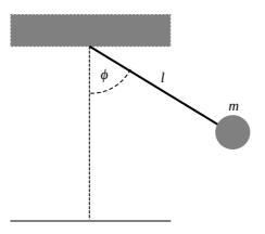
Figure 11.2: A schematic figure illustrating configuration of the pendulum, to determine gravitational acceleration,  $g_E$ , at Earth's surface.
